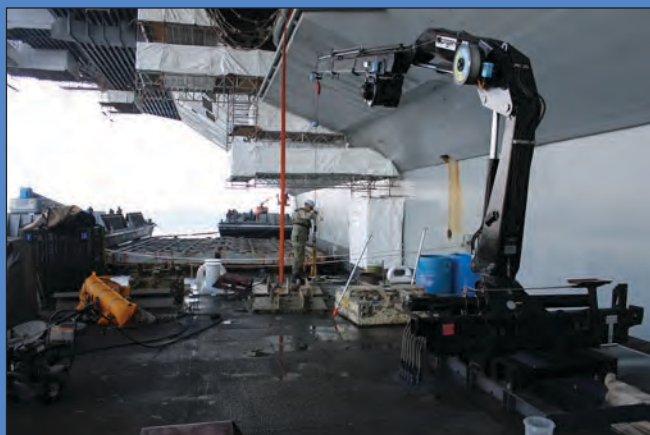
ND1 Buzek supervises Morgan Crane lift of cofferdams on USS RONALD REGAN. (Photo by ND1 Trautman)
