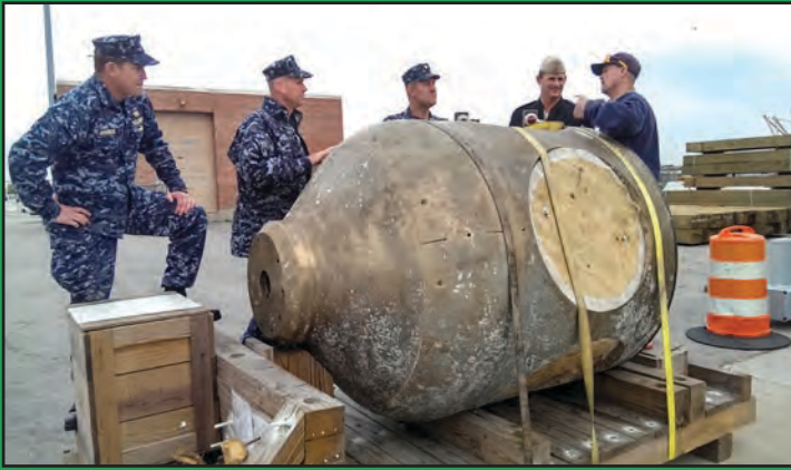
NAVSEA 00C Technical Expert Bill Reid (right) explains to Carrier Strike Group 12 commander Rear Adm. Andrew Lewis how the hub of USS Forrest Sherman (DDG 98) fits into the cofferdam during MARMC divers' hub change out.
